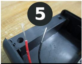
5- Use a knife or your cutting tool to strip the insulation off the wires, about 10mm
