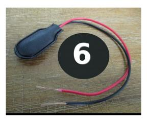
6- Do the same to the two wires on the new clip. Strip back about 10mm
