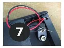
7- Twist the wires together. Red to Red and Black to Black. Make sure the twisted joints of each colour do not touch each other. Keep them separated.
