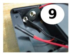
9- Wrap the cut pieces of insulating tape tightly around each of the twisted joints. Make sure there are no wire strands poking out after wrapping the tape. An extra piece of tape can be wrapped around both the joints to make it into a single joint – might look a little neater!
