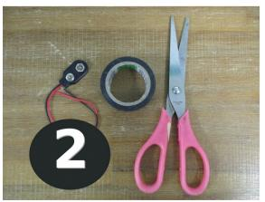
2- You will need a new PP3 clip, insulating tape and a small cutter or scissors will do
