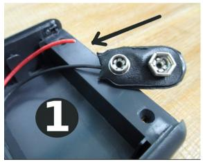
1- Typically one or maybe both wires have broken off
