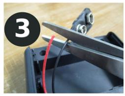
**3-** Use your cutting tool to cut off the old battery clip
